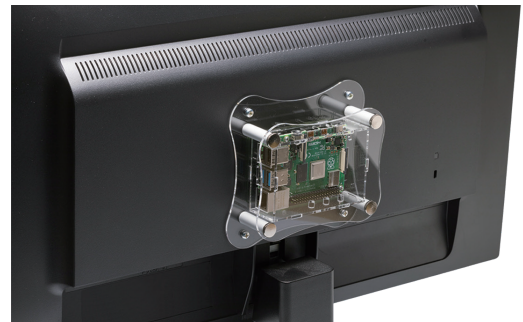
RPA-4B-1F is compatible with VESA Mount Standards (100 x 100mm), and can be installed on the back side of PC displays, etc.
