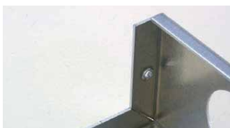
Increasing surface area on a thin metallic sheet for screw threads to bore into.
