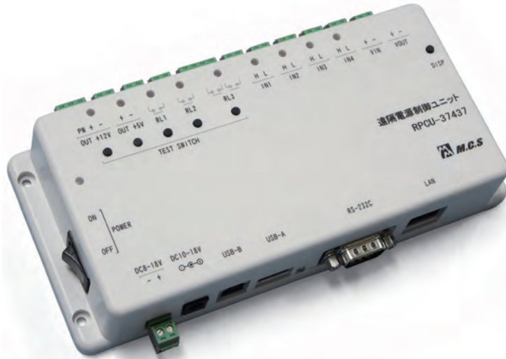
Remote Power Control Unit
